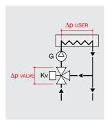
In a mixing circuit, the portion upstream from the three-way valve is usually a zone with negligible  $\Delta$ p (and there is normally a hydraulic separator). Therefore the main pressure drop is due to the three-way valve, giving it regulating authority. For this reason, the three-way valve can be dimensioned by considering an acceptable pressure drop for the user circuit pump, which indicatively may be from 5 % to 15 % of the pressure drop in the user circuit:
